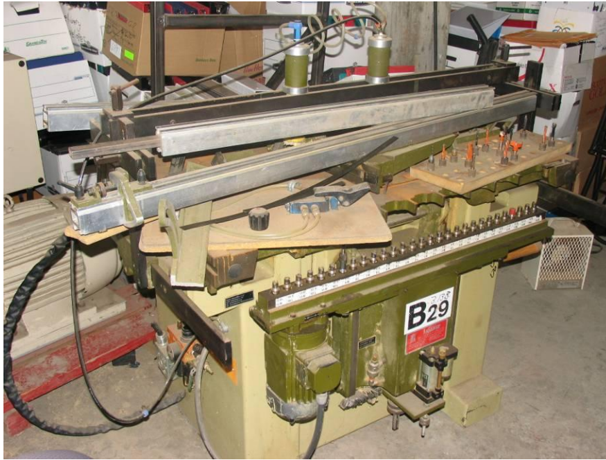
Parcel 3.13B ZANCHERI & BOSCHETTI Multi-Bore 29 Spindle, B295, s/n B49989
