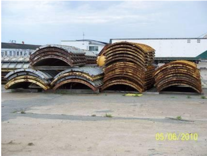
Parcel 3.8B EFCO pier-column forms (approx. 80)
