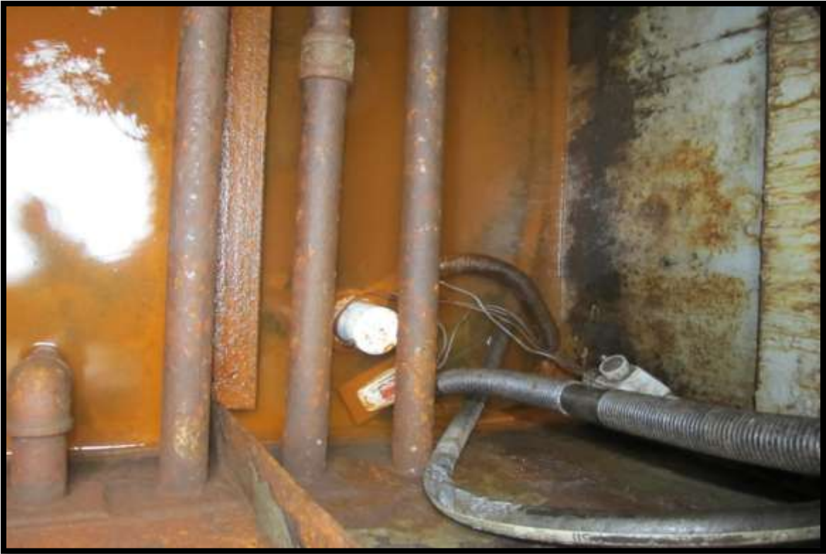
TYPICAL COMOPARTMENT BILGE PIPING
