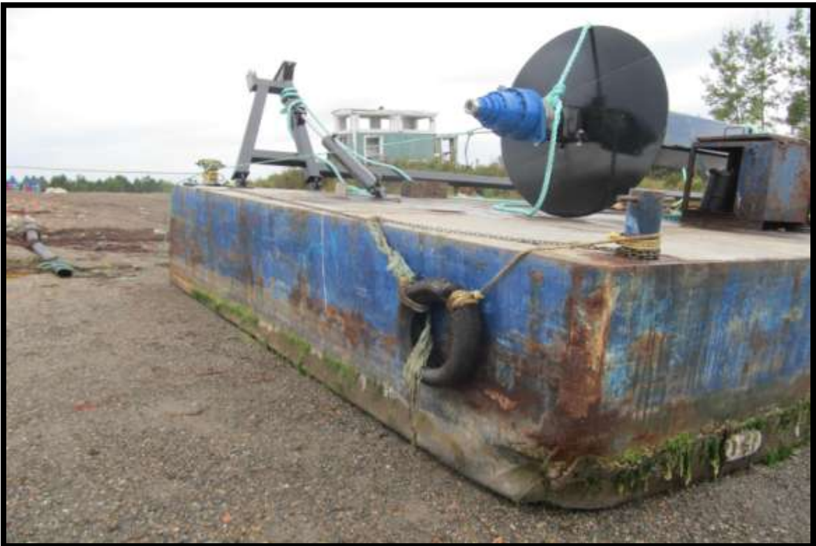
TRANSOM – DAMAGE NOTED ON STARBOARD BOTTOM CORNER
