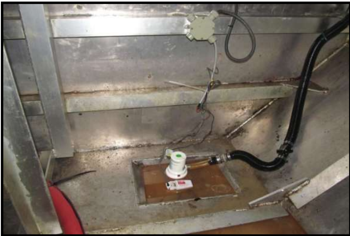
TYPICAL BILGE SUCTION ARRANGEMENT
