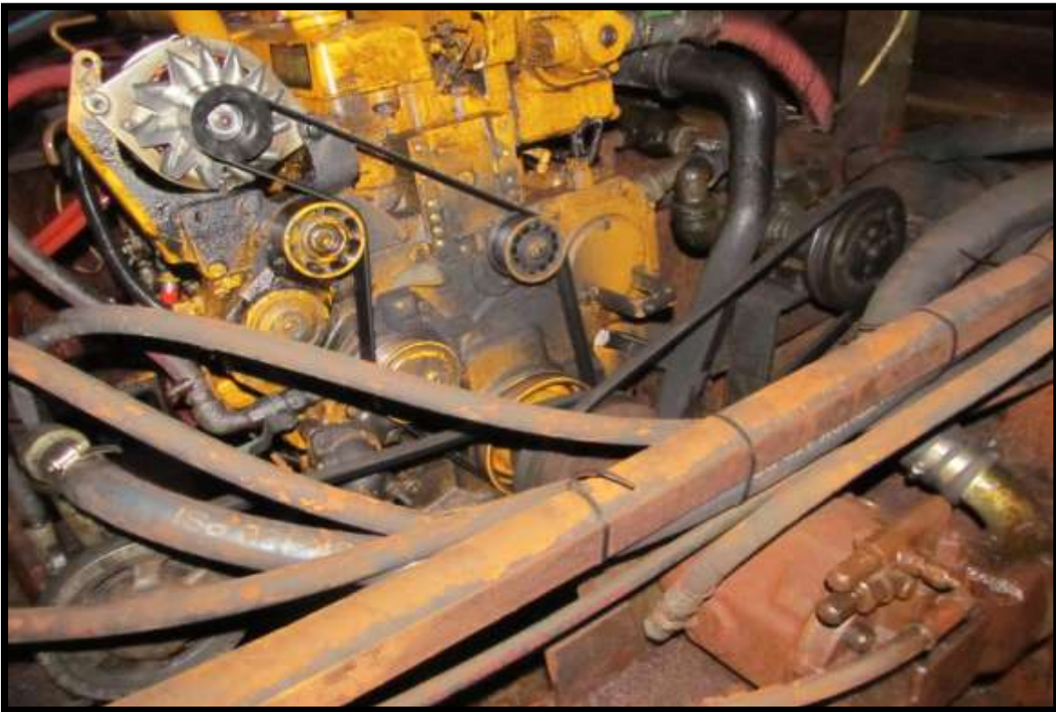
ENGINE FRONT: HYDRAULICS AND WASHDOWN PUMP
