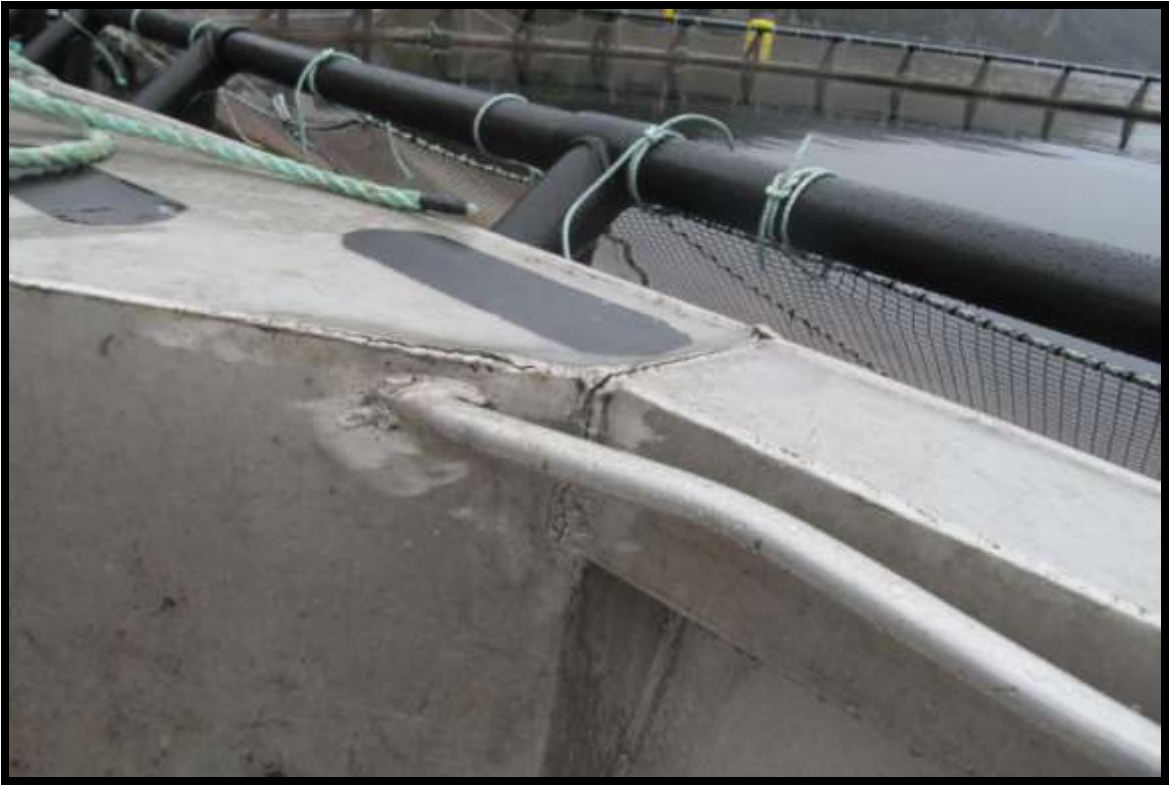
BULWARK WELD FRACTURES
