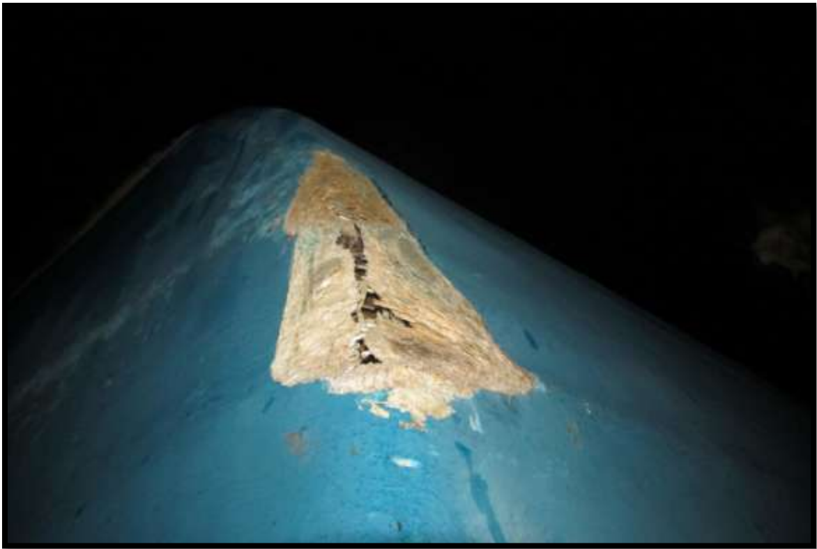
DAMAGE TO STARBOARD SIDE TRANSOM CORNER
