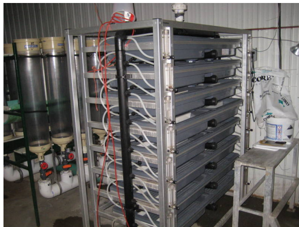
Ref. #45 Comphatch Custom Designed and Fabricated Salmon Egg Incubation and Hatching System(New 2014)
