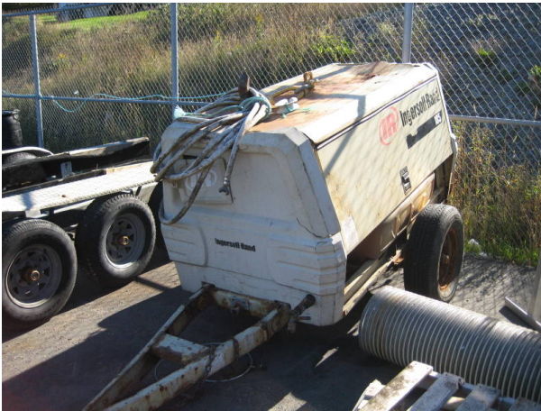
Ref. #133 Ingersoll Rand Model PA185, 185-CFM Portable Trailer Mounted Air Compressor, S/N 7827AW (New 2001)
