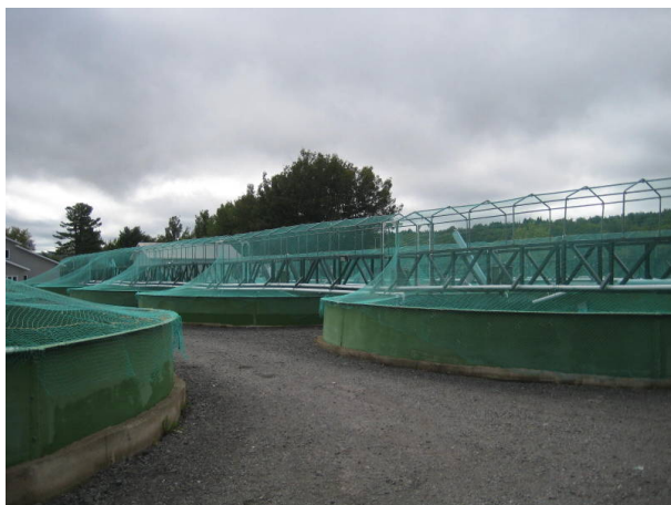
Ref. #23 40' Dia. x 6'H, 200-Cu. Meter Fiber Glass Tanks
