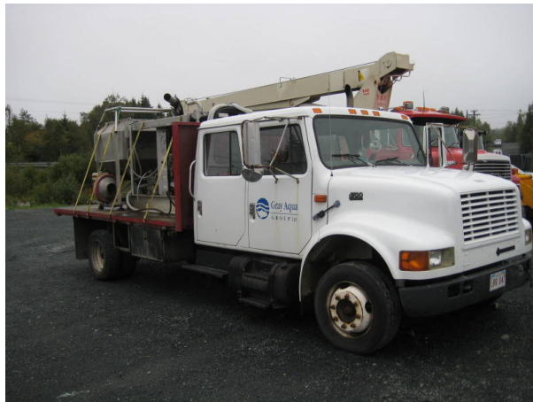
Ref. #108 International Model 4700-T444E, 12' Crew Cab Single Axle Flatbed Truck, S/N 1HTSLADM74H245447 (New 2004)
