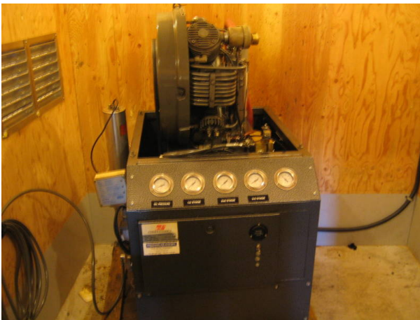
Ref. #137 EP 6,000-PSI Dive Tank Compressor(New 2012)
