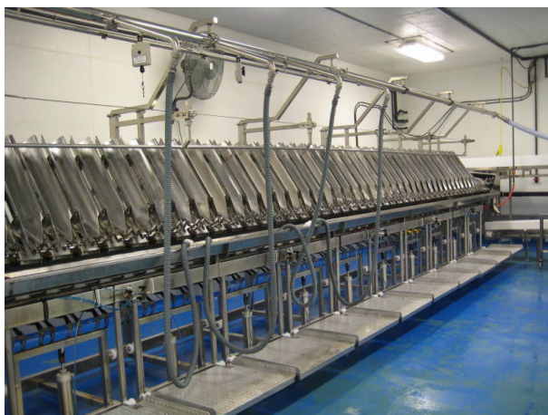
Ref. #152 Marel 40'L Stainless Steel 10-Station De-Heading and Gutting Line, S/N 19940-007
