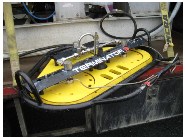
Ref. #105 MPI Model Terminator 3, 3-Head Net Washer(New 2011)
