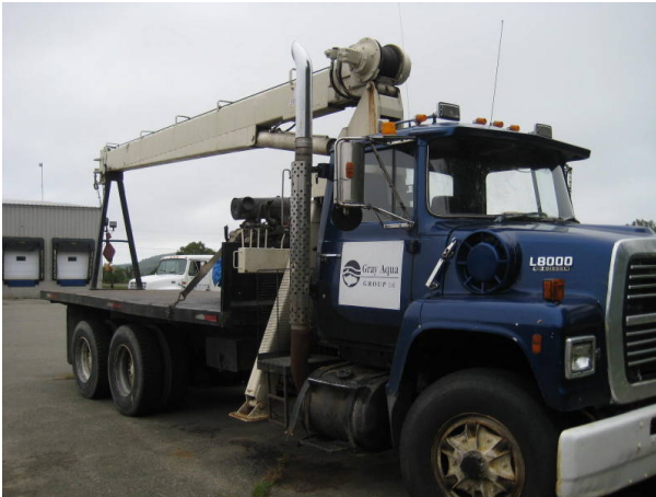
Ref. #75 Ford Model L8000, Diesel Tandem Axle Boom Truck Crane, S/N 1FDZW82A1JVA45247 (New 1988)
