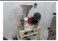
**EXTRACTION** - KannaMill Schutte Hammermill MM-12 Food Grade Mini Mill, w/ Vacon X Series X4C1S010C Variable Frequency AC Drive, Weg Motor.
